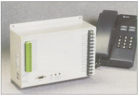
contacts or thermistor inputs in any combination. These remote monitoring systems also have the ability to count pulses, totalize and measure RPM's. Outputs can manually or automatically switch heavy loads.
